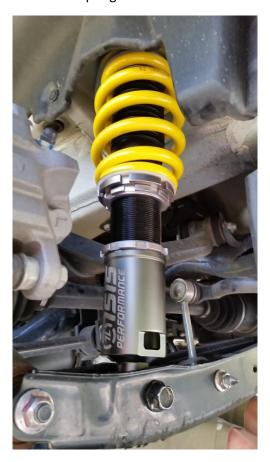
Insert the ISIS Performance Coilover and thread the 2 top nuts. Align the bottom and jack up the lower control arm and make contact, jack the lower control arm up and down a few times till the bottom mount is in place with the holes in the LCA and push in the bolt. It's a tight fit, that's the way its supposed to be, it will fit.
