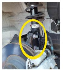
Take the nuts off the bolts that connect the shock to the knuckle and remove the nut that connects the sway bar end link from the bracket on the shock. (Do this on both sides to release tension to help the endlinks to be remove and install easier)
